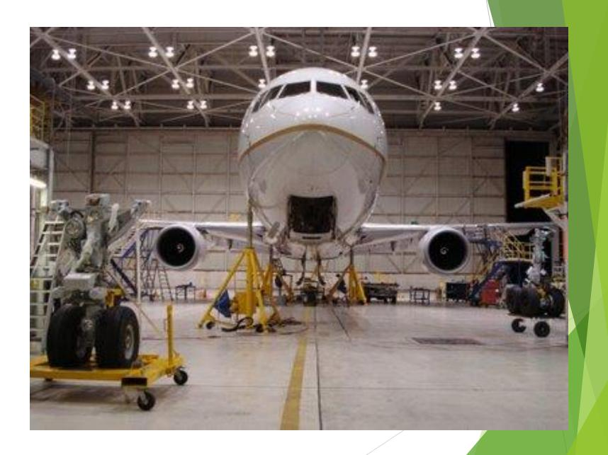
▶ Before releasing jack pressure and lowering the aircraft, make certain that all cribbing, work-stands, equipment, and persons are clear of the aircraft, that the landing gear is down and locked, and that all ground locking devices are properly installed.
